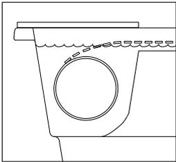
The underwater standard slat system can be installed in pools from our Monaco and Antibes ranges. The standard set includes a 140 Nm-24-IP68 fiberglass roller with pool-wall fixings, a motor control key box, a fixing kit for roller tube straps, and a 110 x 65 mm aluminium beam for top-down wood support. This cover system works with standard, 10–12 cm water-level systems.
