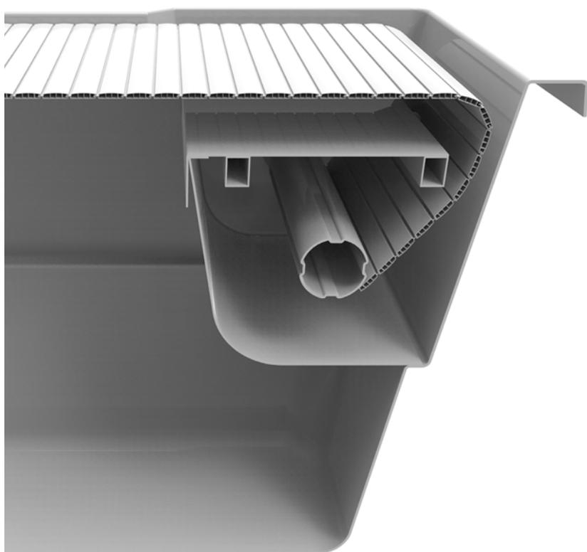
The underwater bench slat system can be installed in pools from our Monaco and Antibes ranges. The standard set includes a 140 Nm-24-IP68 fiberglass roller with pool-wall fixings, a motor control key box, a fixing kit for roller tube straps, and a 110 x 65 mm aluminium beam for top-down wood support. This cover system works with both standard and high water-level systems. The submerged bench above the slat system works perfectly as a sun deck.
